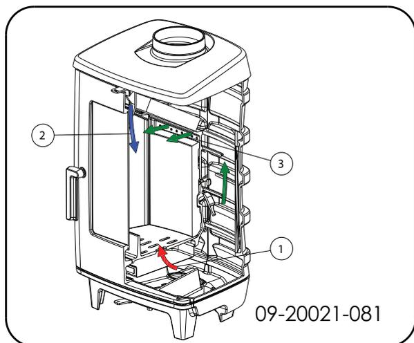
The primary air inlet regulates the air under the grate (1).
