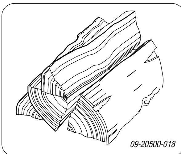
If the logs are stacked tightly, the wood will burn more slowly as the oxygen can only reach some logs easily. If you want to burn wood for a longer period, make a compact stack.
