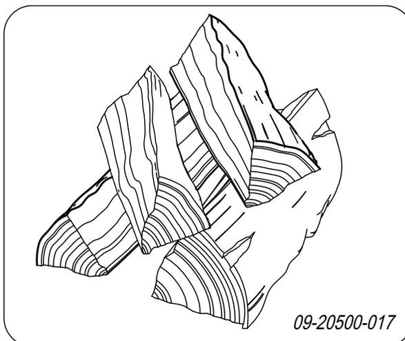
If the logs are stacked openly, the wood will burn quickly as the oxygen can reach each log easily. If you want to use the stove for a short while, make an open stack.
